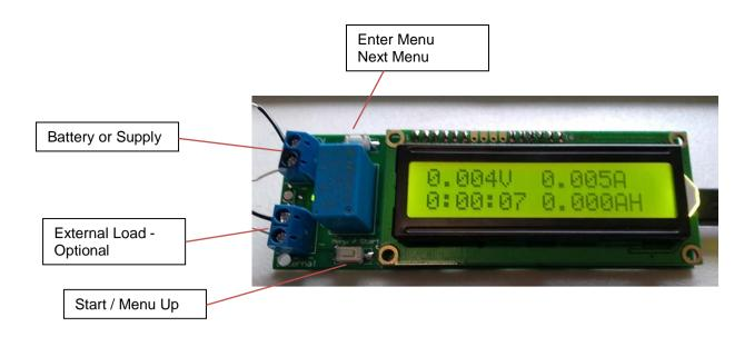
The + and – connections are clearly shown on the board. Reverse connection is unlikely to cause damage, but the circuit is not short circuit protected and it may be damaged if the external load connector is short circuited so please take care.
