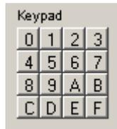
The hex keypad simulates a 4x4 hex keypad with 4 rows and 4 columns. Key 0 is row 0, column 0, Key 1 is row 0, column 1 and so on up to Key F which is row 3, column 3. When a key is pressed with a mouse the device connects the input to the output. If the key is held down with the mouse then it will remain pressed.
